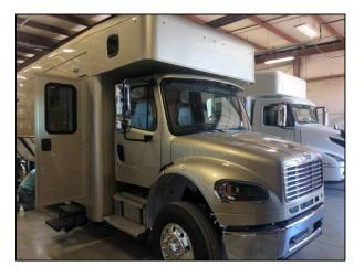
The Freightliner M2-106 chassis is designed for optimum power and performance with 350HP / 1,150 lb-ft and Allison transmission.
